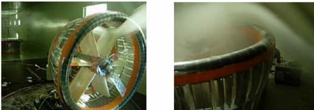
Figure 8: Rotor flow visualisation in a wind tunnel in vertical (a) and horizontal flight (b)
